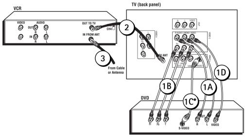
\* If you connect an S-Video cable, you must connect the audio cables to the VIDEO 1 AUDIO jacks on the back of the TV, <u>not</u> the VIDEO 2 AUDIO jacks.
